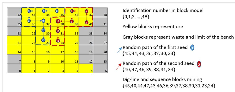
Figure 2 - Selection scheme of blocks for two shovels and seven blocks per each shovel.
