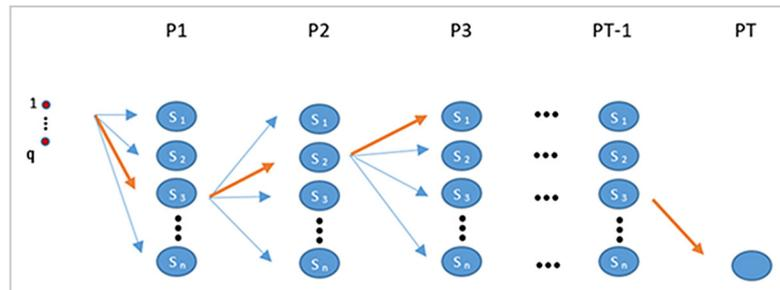
Figure 3 - Sequence adopted to select the mining advance within each dig-line.
