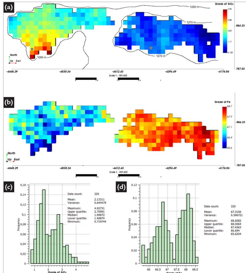
Figure 4 - a) Maps of reference grade model for  $SiO_2$ , b) maps of reference grade model for Fe, c) histogram and statistic for  $SiO_2$ , d) histogram and statistic for Fe.
