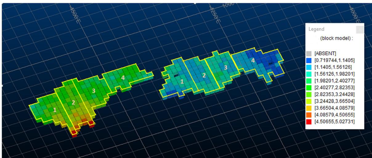
Figure 8 - Dig-lines 1, 2, 3 and 4 manually drawn on the SiO<sub>2</sub> block model.
