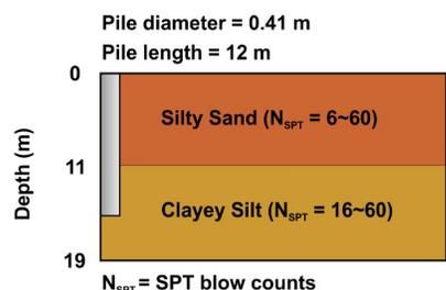
Figure 8. Soil profile at Site D (test pile P7).
