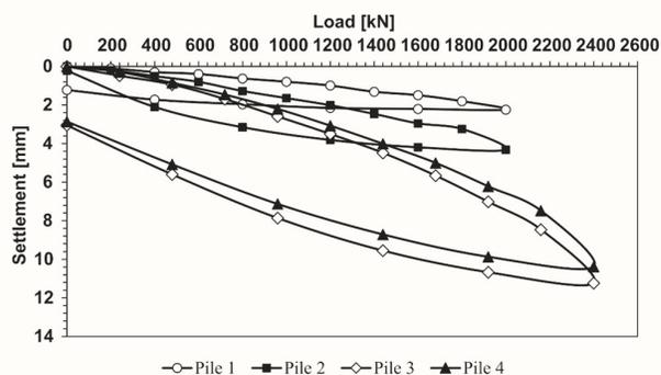
Figure 10. Results from static load tests for piles P1, P2, P3, and P4.
