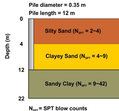
Figure 6. Soil profile at Site C (test pile P5).
