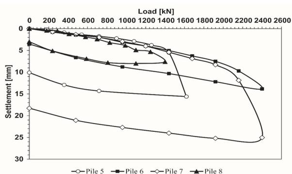
Figure 11. Results from static load tests for piles P5, P6, P7, and P8.
