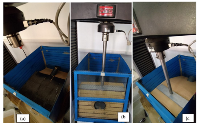
Figure 5. (a) A carbon fiber layer being installed within the slope; (b) rear view; (c) top view.
