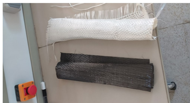
Figure 2. Fiber glass and carbon fiber elements used in this study.
