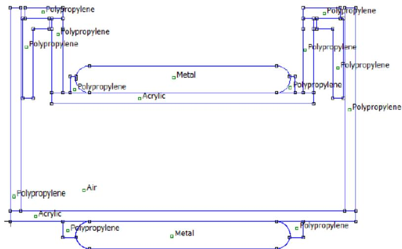
**Figure 1.** Sectional view of the post-filling electro-pasteurization tunnel. Having as dimensions: width: 646 mm, Height: 400 mm; Electrodes (50 mm x 400 mm).
