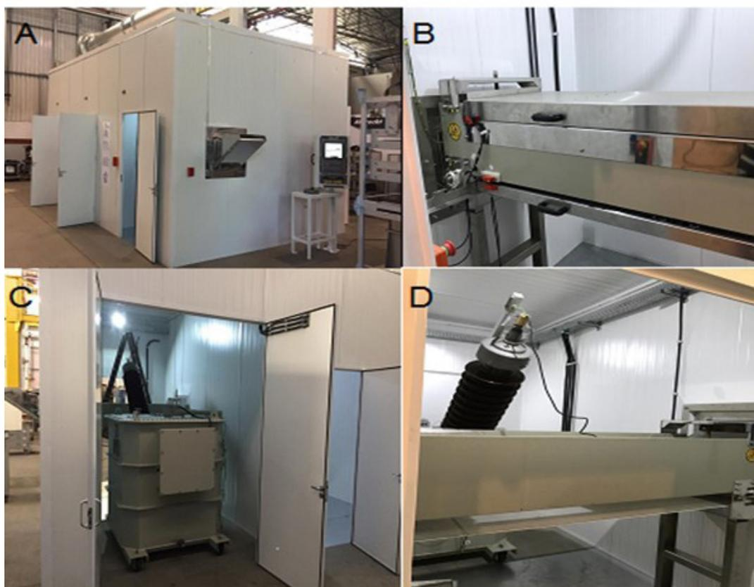
**Figure 4.** PEF industrial-scale apparatus showing: A) chamber with automated control panel; B) isolated treadmill for pasteurization of packed foods; C) electrical font; D) coil with ceramic insulation on the treadmill.
