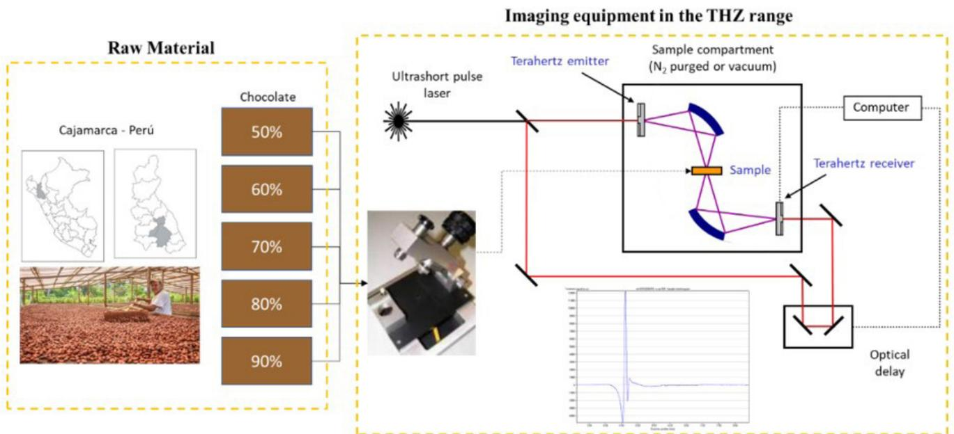
Figure 1. Terahertz pulsed spectroscopy operation schematic.
