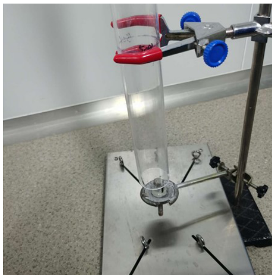
Figure 1 - Modified BIM-IV bio-impact machine (250-g metal ball).
