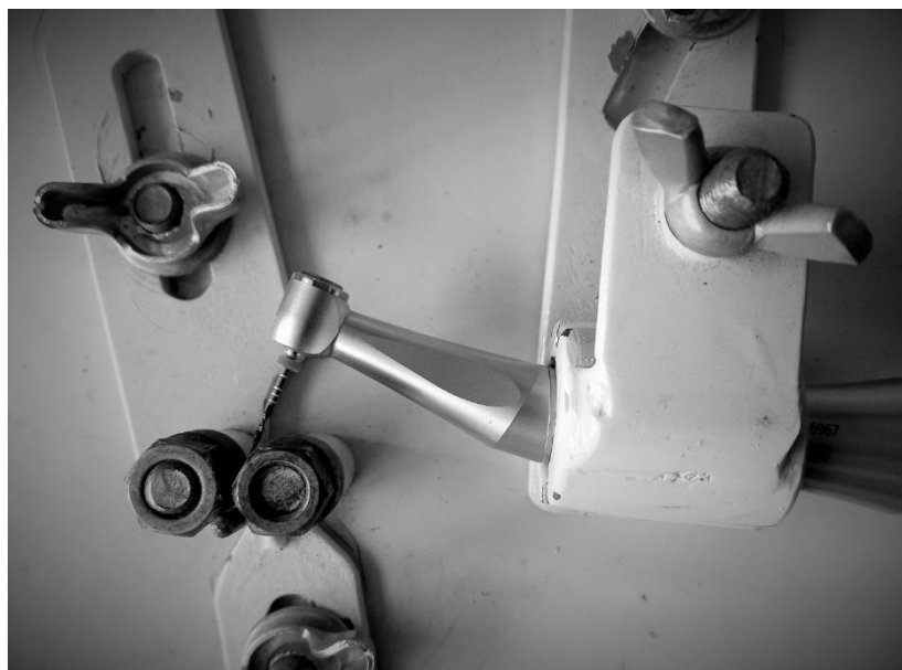
Figure 2. Cyclic fatigue resistance test
