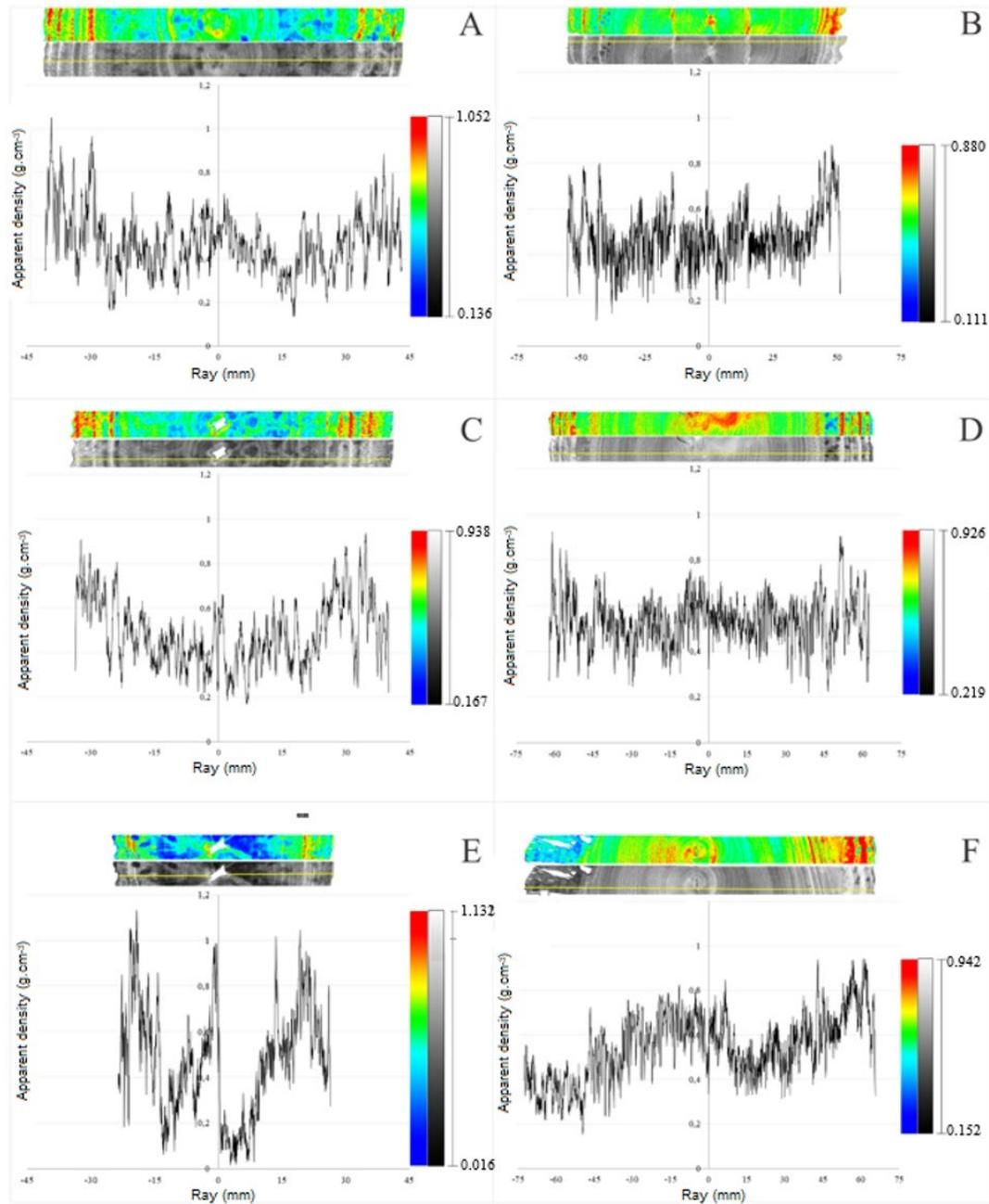
**Figure 7:** Profile of the apparent density at 365 days of storage in the wood of *Eucalyptus* samples with a lower diameter class in the upper (7a), intermediate (7c) and bottom (7e) regions, respectively, and a higher diameter class in the upper (7b), intermediate (7d) and bottom (7f) regions, respectively.
