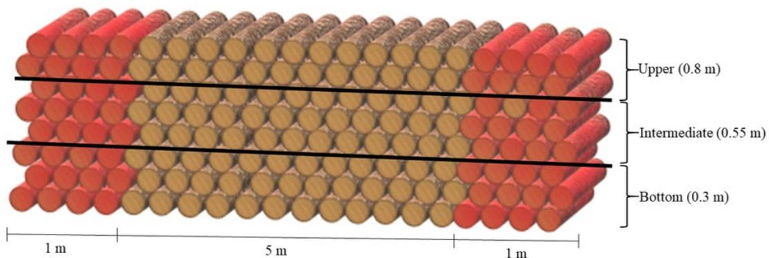
**Figure 1:** Scheme with the dimensions of the pile of eucalyptus wood logs with those marked with red disregarded in the sampling.
