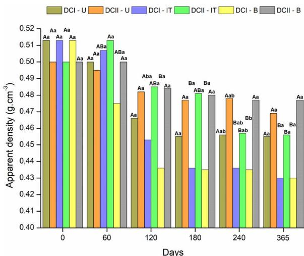
\*The uppercase letters analyzed the differences between days, and the lowercase letters analyzed the differences between the diameter classes (DC) of the logs associated with their positions in the pile, each storage period. Values followed by the same letter (upper or lower case) per bar do not differ from each other using the Kruskal-Wallis test at 5% probability.
