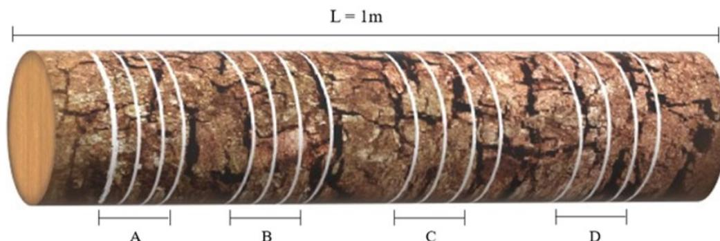
**Figure 3:** Sectioning position to removing the discs in the longitudinal direction of the logs to assess their density.
