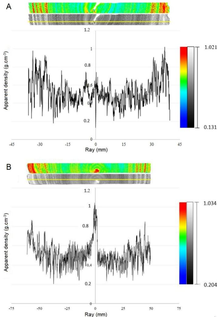
**Figure 6:** Profile of the apparent density of *Eucalyptus* samples with lower (a) and higher (b) diametric class on day 0 of storage.
