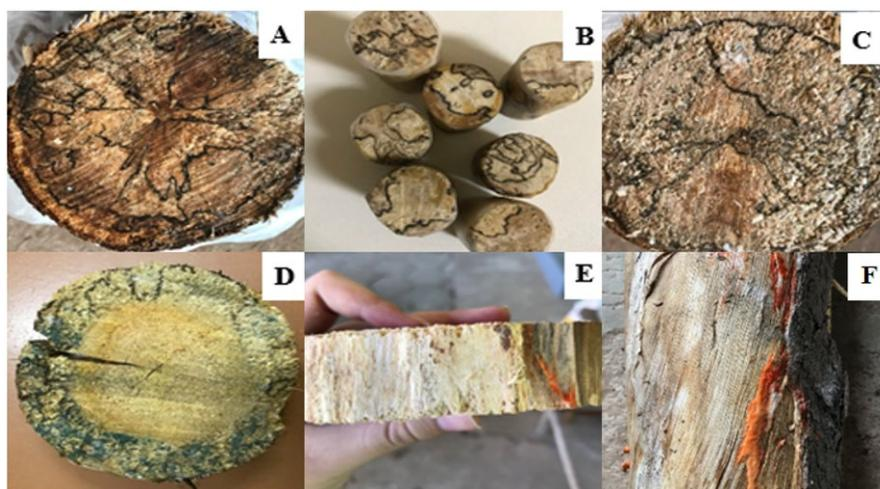
**Figure 5:** *Eucalyptus* woods at 365 days of storage with signs of white (5a, 5b, 5c and 5d) and soft (5d), spalted wood (5a, 5b, 5c and 5d), and apparent defibrillation (5e and 5f).
