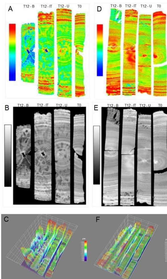
**Figure 8:** Samples at 0 (T0) and 365 (T12) days of storage of wood with smaller (DCI) and larger (DCII) diameter classes with the rainbow (8a and 8d) and gray (8b and 8e) scale and plotting the 3D density variation surface (8c and 8f).
