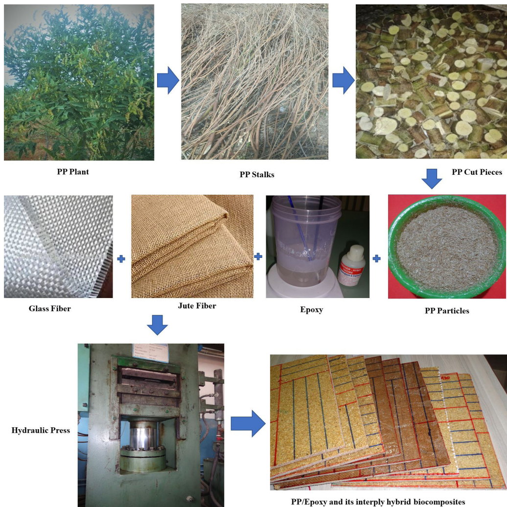
Figure 1. Preparation of PP stalk particles and the development of EP composites and their hybrid composites.
