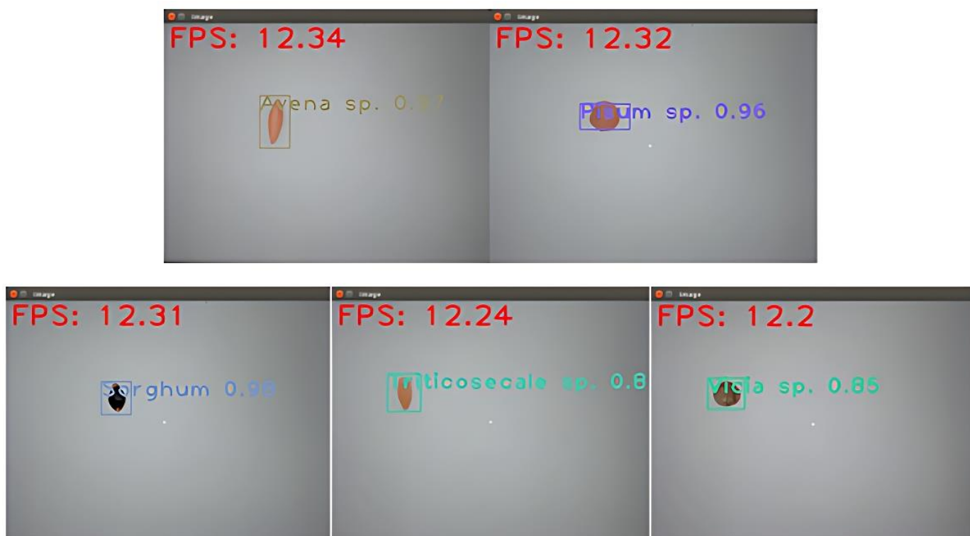
Figure 4. Accuracy and FPS samples of forage crop seeds detection with YOLOv4-tiny model at TX2.
