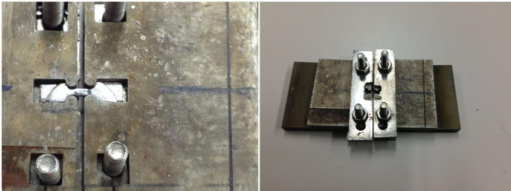
**Figure 3:** The clamping mould in tensile test.
