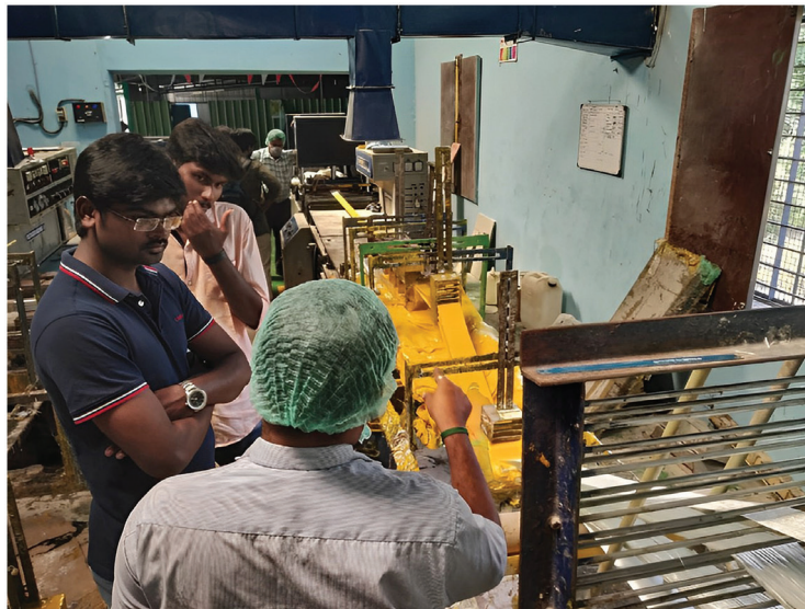
Figure 1: A view on fabrications of GFRP angle sections by pultrusion process.
