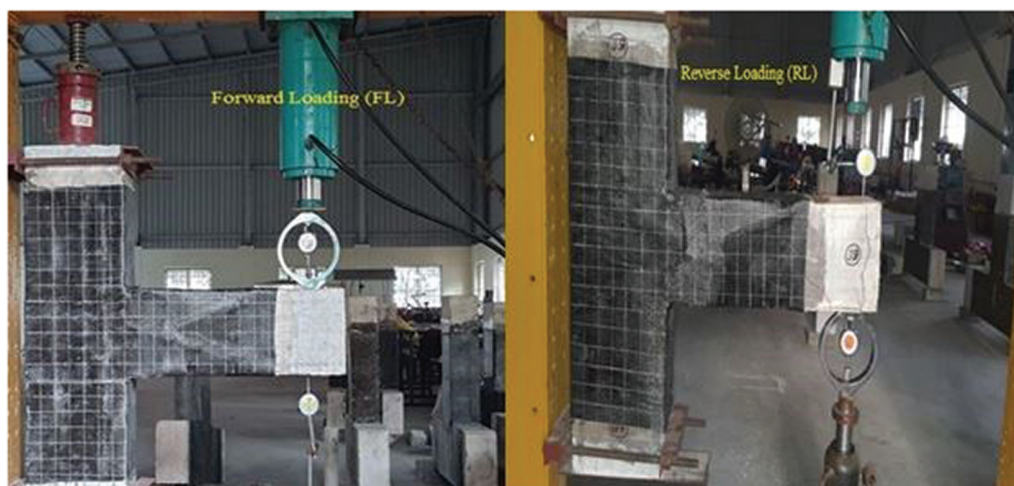
Figure 2: Cyclic load set-up.
