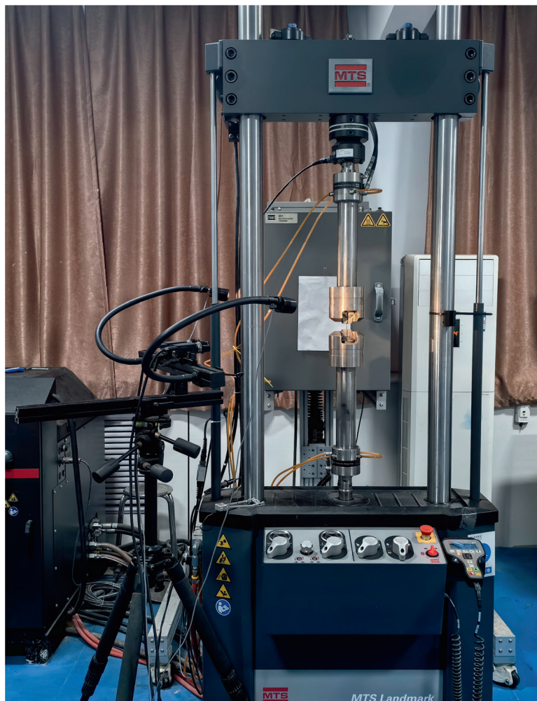
Figure 4: Tensile and DIC test.
