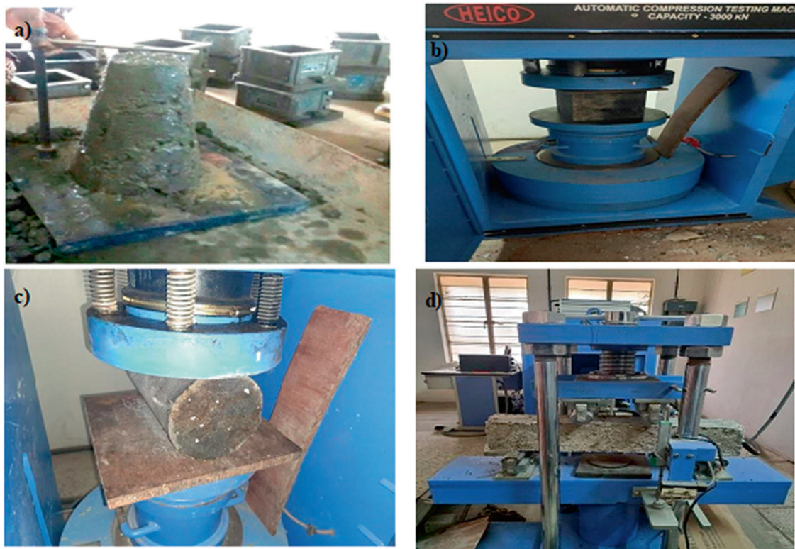
Figure 3: Experimental tests setup. (a) Slump test (b) f_{cs} test (c) f_{sts} test (d) f_{fs} test.
