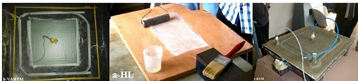
Figure 1: (a) HL based GFRP production, (b) VARTM based GFRP production and (c) RTM based GFRP production.
