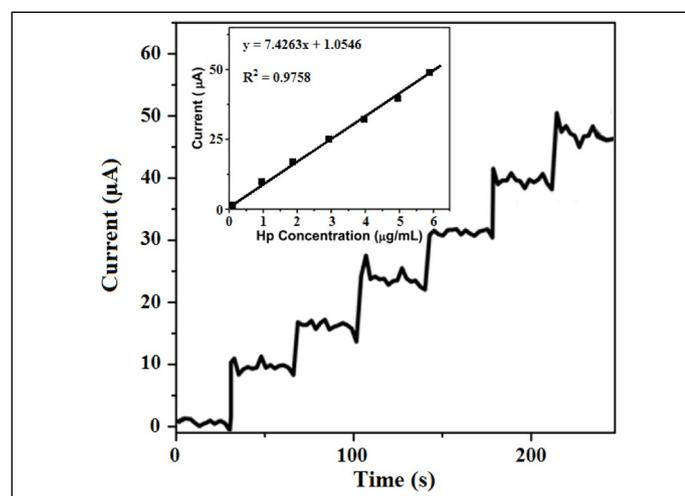
**Figure 3.** (A) Amperometric measurements of gHb-DsDNA/Au/GCE to successive adding 1  $\mu\text{g}/\text{mL}$  Hb into 0.2 M PBS at 0.25 V potential; (B) Inset figure shows the calibration curve.
