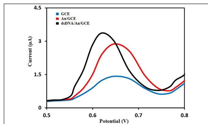
Figure 2. DPVs of GCE,Au/GCEand dsDNA/Au/GCE at 20mV/s scan rate into 0.2M PBS including 10mg/ml Hb.
