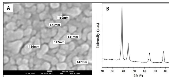
Figure 1. (A) Surface morphology of AuNPs onto GCE and (B) X-ray diffraction pattern of electrodeposited AuNPs.
