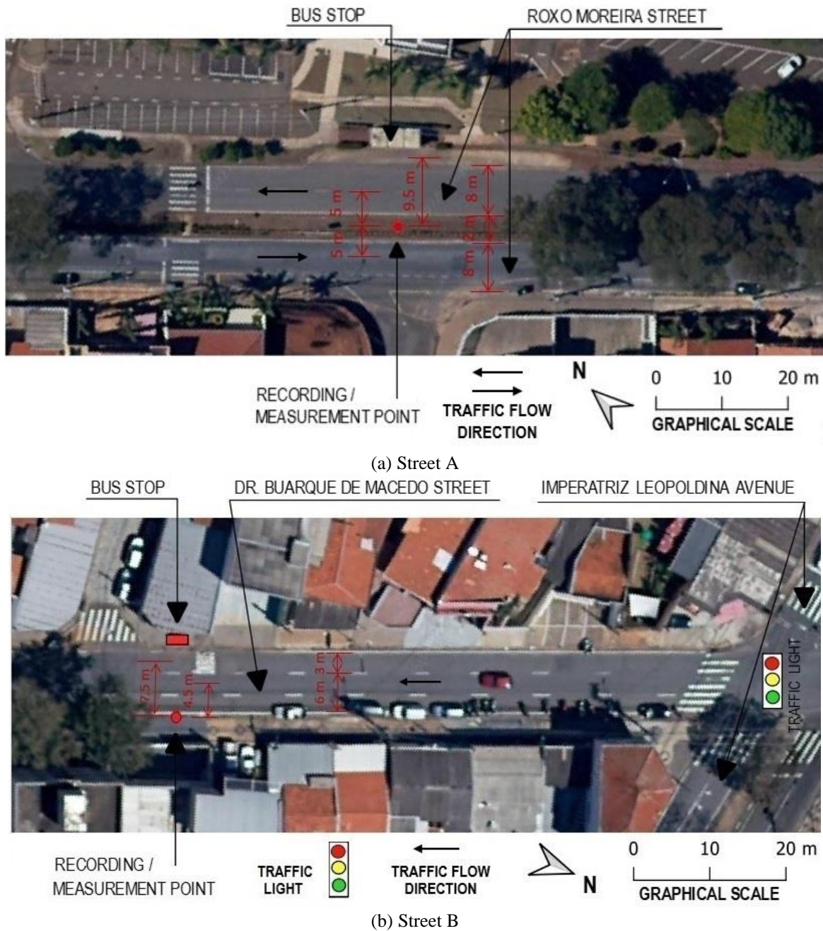
Figure 8 - Position of acoustic recording/measurement points (a) and (b)
