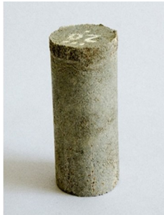
Figure 5. Polymer bonded CS cylinder with PC_g = 20\% .
