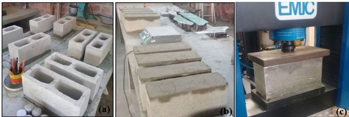
Figure 1. Concrete blocks: a and b) capping c) compressive strength
