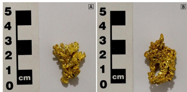
Figure 8. (A) Gold nugget with dimensions of 2.9 cm × 2.3 cm × 1.5 cm and a weight of 15.06 g, crystallized in arborescent habit with a slightly pitted surface. (B) Gold nugget with dimensions of 3.4 cm × 2.3 cm × 1.2 cm and a weight of 26.30 g, xenomorphic, low sphericity, angular geometry, intensely pitted, spongy texture, and presence of voids and cavities, mostly filled with iron oxides/hydroxides.
