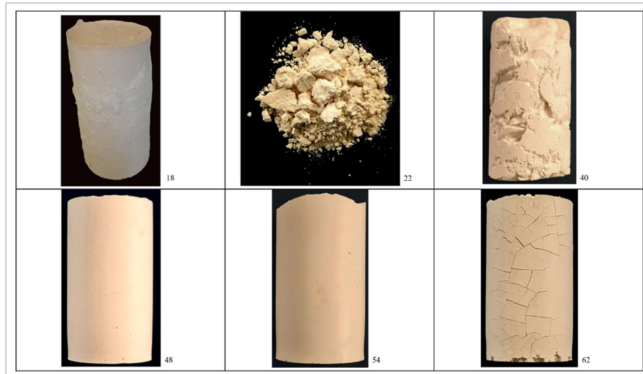
Figure 3 - Pictures of the geopolymer samples, according to the sample number of Table 1.
