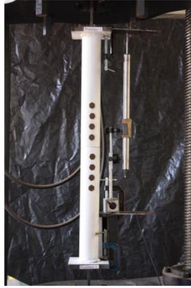
Figure 1 - Sleeve connection with CHS (Roquete, 2018).
