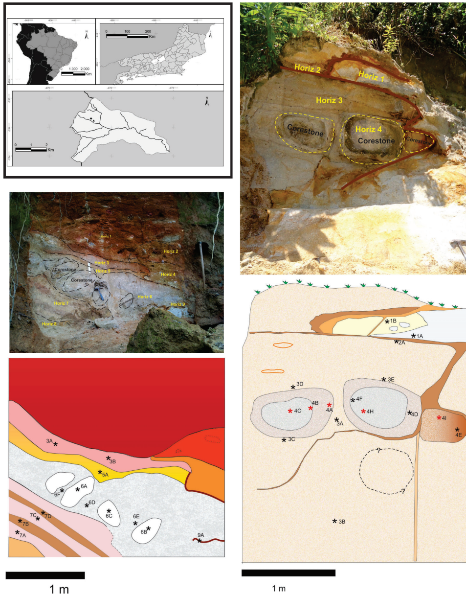
Figure 1. Above location of profiles 1 (triangle) and 2 (cross) in Principe Catchment, Rio de Janeiro State, Brazil. Below photos and sketch of profiles 1 (left) and 2 (right) with horizons, corestones boundaries position (? : sugestion) and samples location. Samples 5A, 6A, 6B, 6C, 6D, 6E, 6F, 7A, 7B, 7C, 7D, 9A (profile 1) and 1A, 1B, 2A, 3A, 3B, 3C, 3D, 3E, 4A, 4B, 4C, 4D, 4E, 4F, 4H, 4I (profile 2) are described in Table I.
