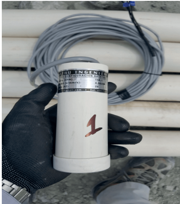
Figure 2. Geophone used in the field test.
