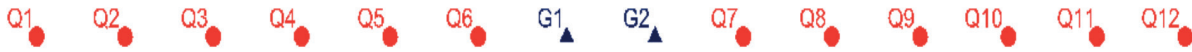
Figure 4. Test configuration where G1 and G2 are the two geophones installed and Q1-12 are the holes with explosive charges.
