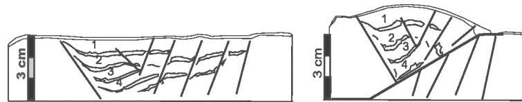
Figure 7 - Line-drawings of the type I sand mica mixture experiment at initial state (i.e. after extension) and after 3.5 cm of shortening to illustrate the layer-parallel shortening process, here shown by layers 1, 2, 3 and 4 near the antithetic border fault.
