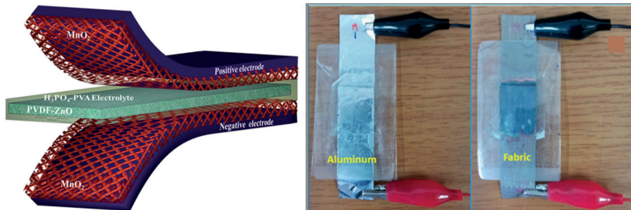
Figure 5 - Piezoelectric self-charging supercapacitor power cell (SCSPC) using MnO_2 nanowires as positive and negative electrodes and a polyvinylidene difluoride (PVDF)-ZnO film as a separator and also a piezoelectric layer (left). Fabricated prototypes using an aluminium foil and a conductive fabric piece as the positive and negative electrodes (right). Modified with permission from Ramadoss et al. (2015). Copyright 2015 American Chemical Society.
