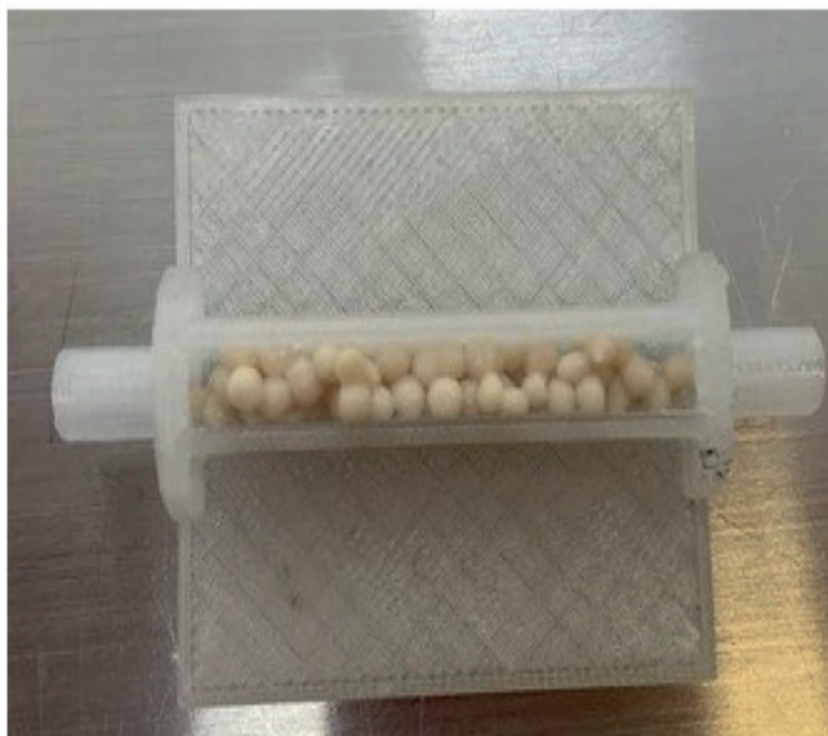
Figure 1. 3D printing microbioreactor filled with 0.7g of S. cerevisiae / S. stipitis immobilizeds, containing 50% yeast S. stipitis and 50% yeast S. cerevisiae .
