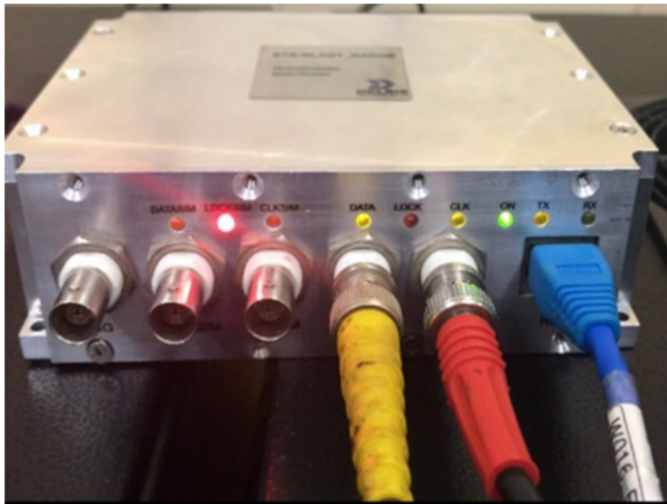
Figure 1. Slant Range device, used to measure the distance between the payload Telemetry Station and the Telemetry Station.
