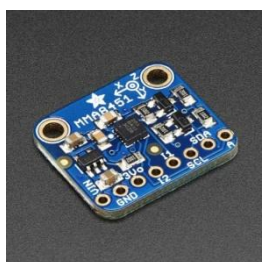
Figure 4. Triple-axis accelerometer/tilt sensor (3-axis..., 2021).
