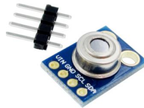
Figure 2. MLX90614ESF-BAA infrared thermometer (Thermal..., 2022).
