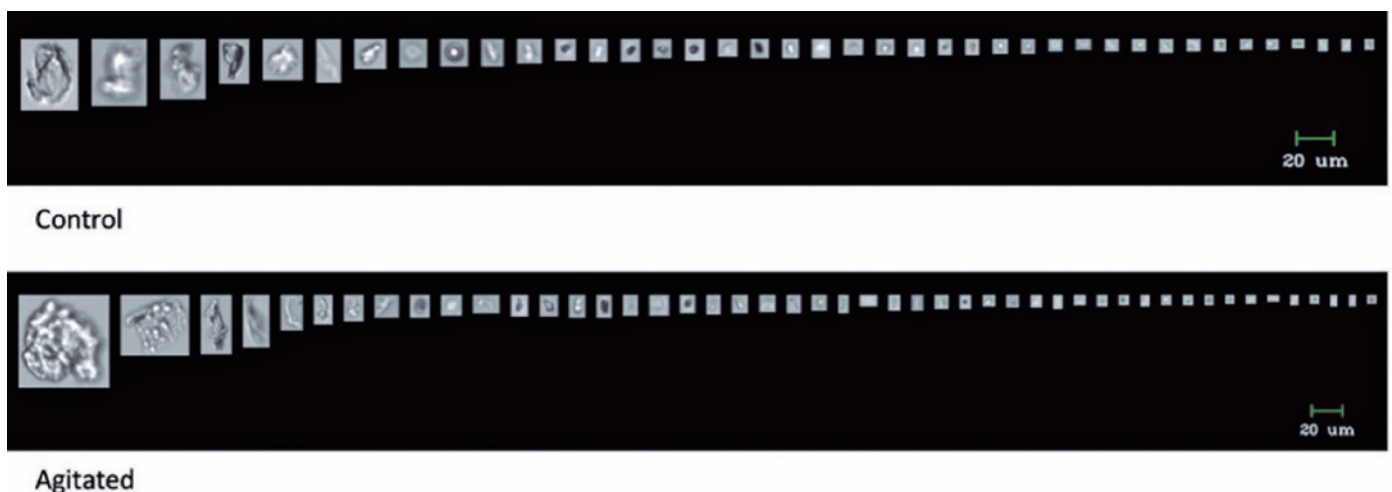
Figure 6. An image of the released particles in the control and agitated groups with the HSW syringe.
