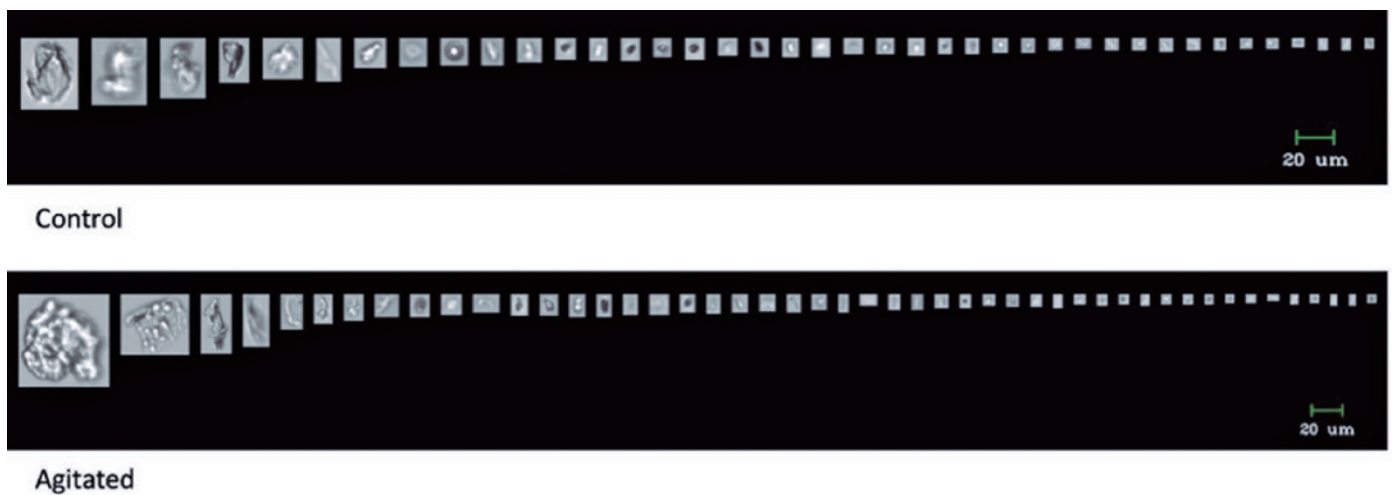
Figure 5. The image of the released particles in the control and agitated groups using the BD Ultra-fine syringe.
