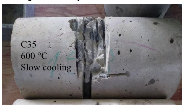
Figure 6 - Concrete embrittlement: emphasis on the transition zone between paste and aggregate in C35 concrete heated to 600 degrees and slowly cooled
