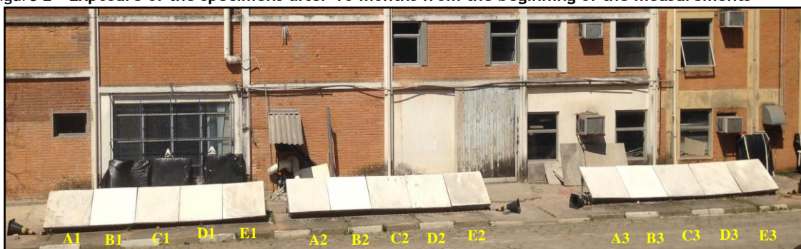
Figure 2 - Exposure of the specimens after 16 months from the beginning of the measurements
