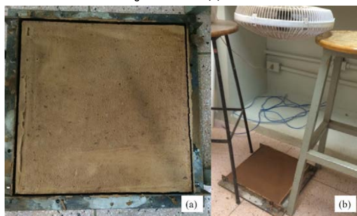
Figure 3 - (a) Restrained volumetric shrinkage test; and (b) Test with airstream
