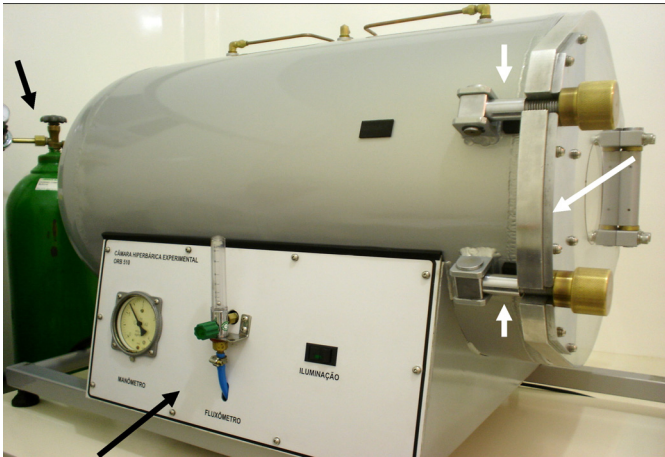
FIGURE 3 – Lateral view of the hyperbaric chamber showing the cover (white long arrow) closed with security latches (short white arrows) and the control panel (long black arrow). In the posterior part, the oxygen cylinder is distinguished (short black arrow)
