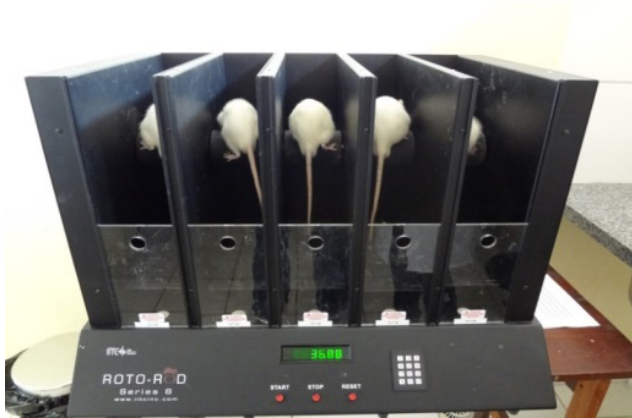
FIGURE 1 - Animals in forced ambulation in Roto-rod (model IITC Life Science, CA, USA).
