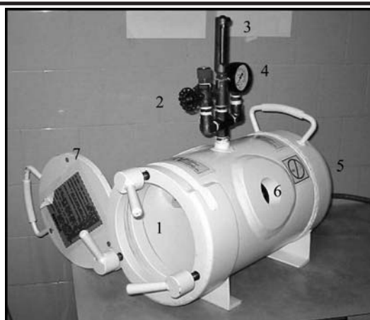
FIGURE 1 - Hyperbaric chamber of cylindrical capsule shape built from carbon steel. 1- Entrance and outlet of the chamber; 2- Oxygen escape valve; 3- Thermometer; 4- Manometer; 5- Tube for oxygen entrance into the chamber; 6- Viewer for the observation of animals within the chamber; 7- Chamber occlusion lid. The chamber is 27 cm wide, 25 cm long and 1,5 cm thick.
