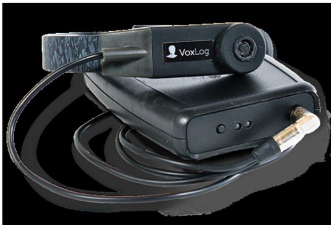
Figure 1. VoxLog® brand 3.1 model Sonvox vocal dosimeter
