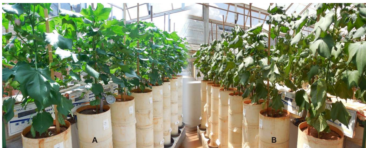
Figure 1. Soil columns on digital scales with cotton plants under well-watered conditions (A) and under water stress (B) at the SITIS phenotyping platform.
