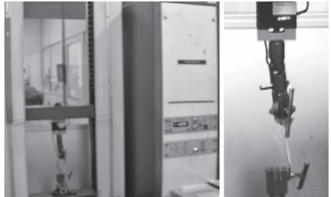
Figure 2 – Photo of the Kratos 500/2000 series 5197 apparatus with 490 N load cell
