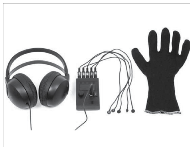
Figure 1. Components of the sensory glove model: headphones, circuit housing and fabric glove.
