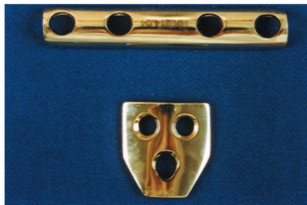
Figure 1 – The two implants used in this investigation, the semitubular plate at the top and the new developed implant at the bottom.
