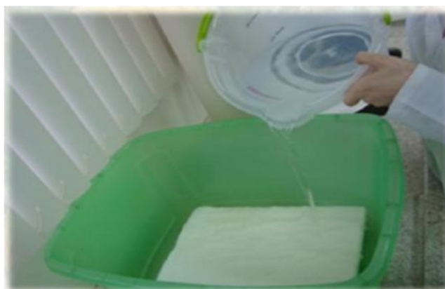
Figure 3. Germitest® paper moistened with water in a ratio of 1:2.5.
