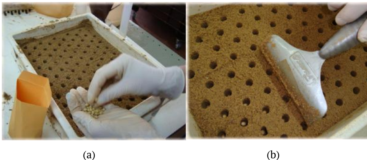
Figure 4. Emergence sand test (a) seed placement and (b) preparation of the carton.
