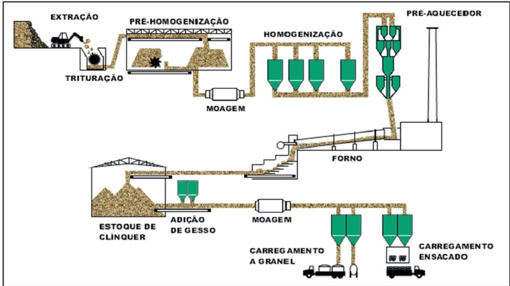
**Figure 1: Cement Manufacturing**
