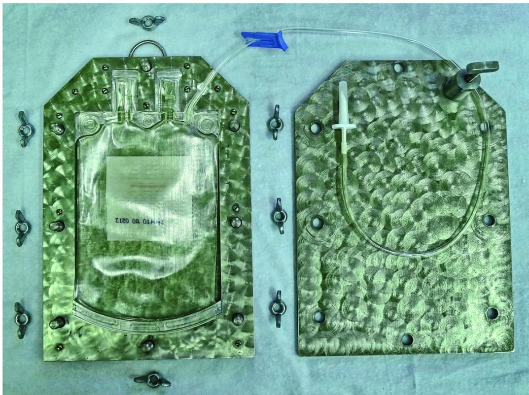
**Figure 1.** Portable, pressure-resistant container with a plasticate container inside for cell suspensions.
