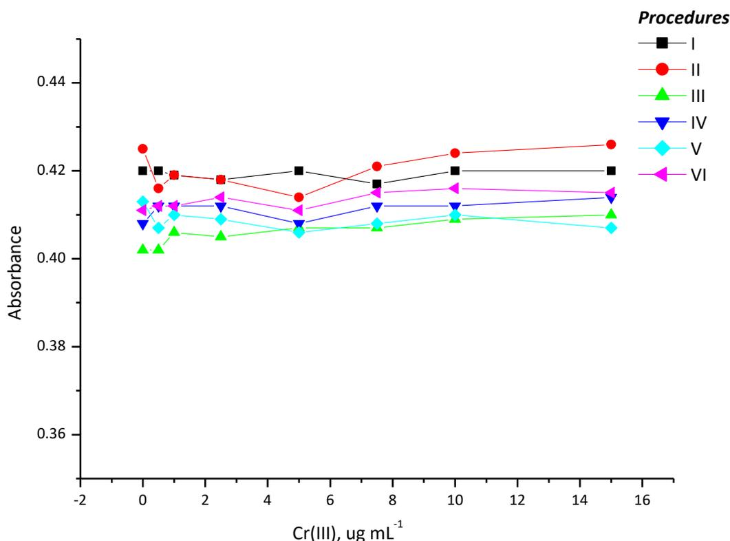
**Figure 4.** Effect of added Cr(III) in different extraction media. Standard of 0.5 µg mL<sup>-1</sup> Cr(VI) spiked with varying concentrations of Cr(III) and subjected to extraction procedures I to VI.
