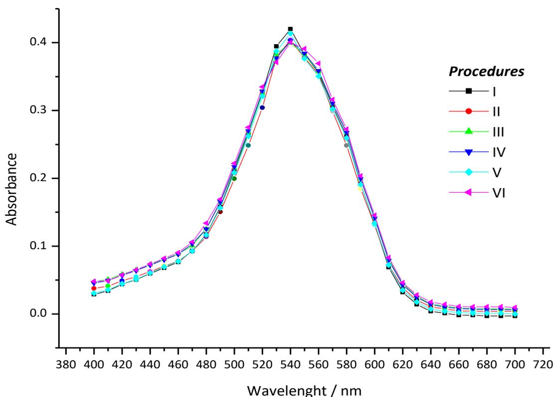
**Figure 2.** Effect of various Cr<sub>2</sub>O<sub>3</sub> pigment extraction media on absorbance band structure. Each solution was spiked with  $0.5 \mu\text{g mL}^{-1}$  Cr(VI).
