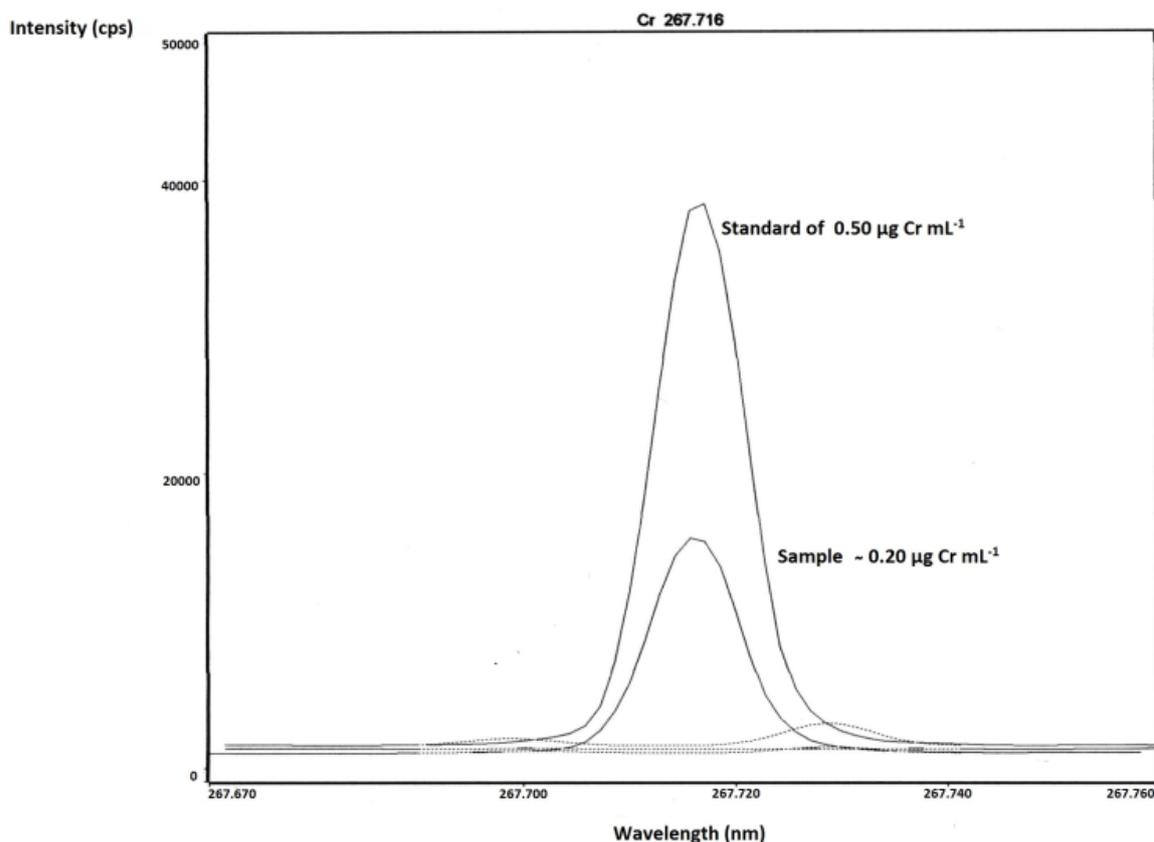
**Figure 1.** Emission spectra generated by introduction of a sample solution prepared using Procedure (II) and a  $0.50 \mu\text{g Cr mL}^{-1}$  calibration standard. Dotted lines reflect procedural blanks; that with a peak at 267.73 nm arises from a processed sample.
