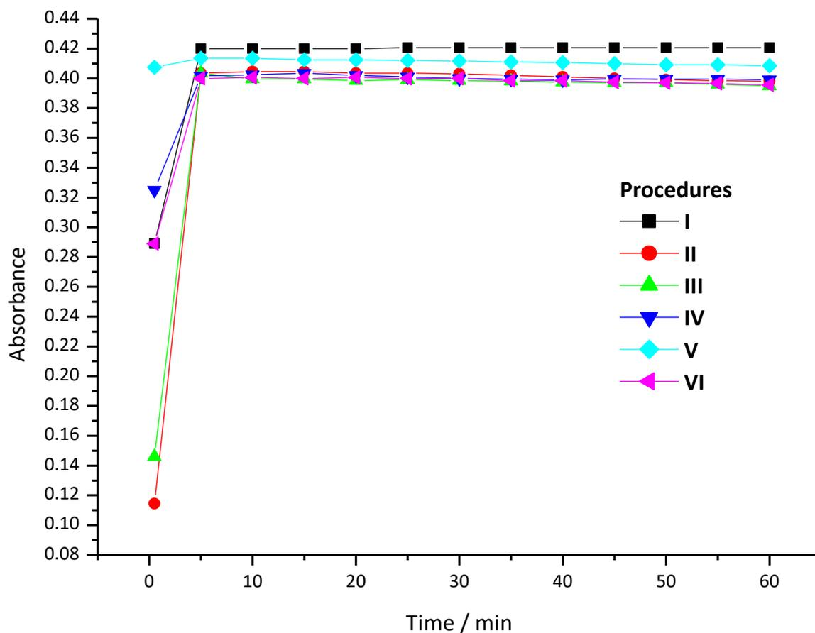
**Figure 3.** Effect of time on development of the [CrDPCO]<sup>+</sup> complex. Different procedural media spiked with 0.5  $\mu\text{g mL}^{-1}$  Cr(VI).
