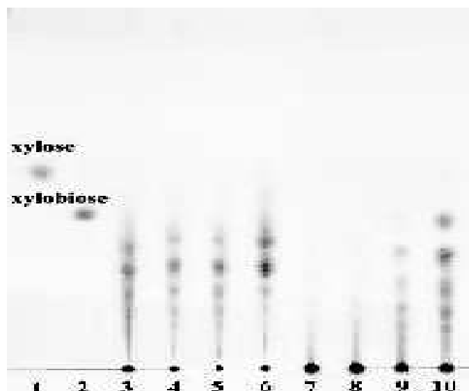
Figure 5 - Chromatographic profile of hydrolysis products of birchwood xylan in pH 6.0 (lines 3 to 6) and 9.0 (lines 7 to 10). Line 1: xylose; line 2: xylobiose; line 3: 10 min.; line 4: 20 min.; line 5: 40 min.; line 6: 120 min.; line 7: 10 min.; line 8: 20 min.; line 9: 40 min.; line 10: 120 min.
