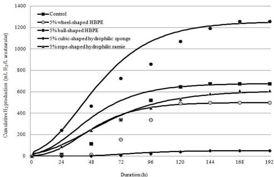
**Figure 2** - Cumulative hydrogen production from vermicelli processing wastewater using immobilizing synthetic and biological materials at 5% (v/v) addition.
