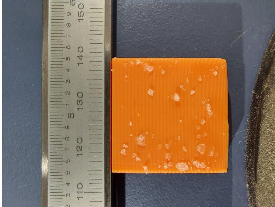
Figure 1. PLA plate coated with the sealant, 24 hours after the application of the varnish and silver nitrate crystals mixture.
