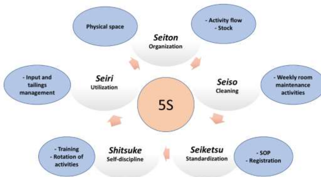
Figure 1. Application of the 5S methodology in the management of the cell culture laboratory. The concepts (Seiri, Seiton, Seiso, Seiketsu, Shitsuke) were mapped according to the activities that must be performed to implement a quality management system that includes disposal, organization, cleaning, standardization, and self-discipline.
